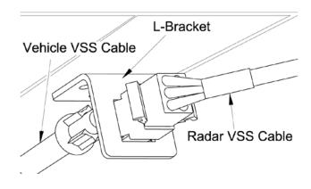
IMPORTANT NOTE: Observe the black polarity marks on the two white 6-pin VSS connectors that plug together. The two white 6-pin VSS connectors can be plugged together with the marks in alignment or the marks opposed. Because of vehicle VSS signal level variations, one of these plug-in positions may not provide a working VSS signal to the radar. If you observe the
