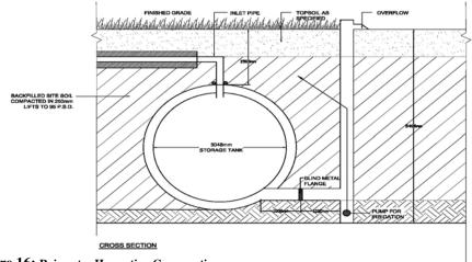
Figure 16: Rainwater Harvesting Cross-section
