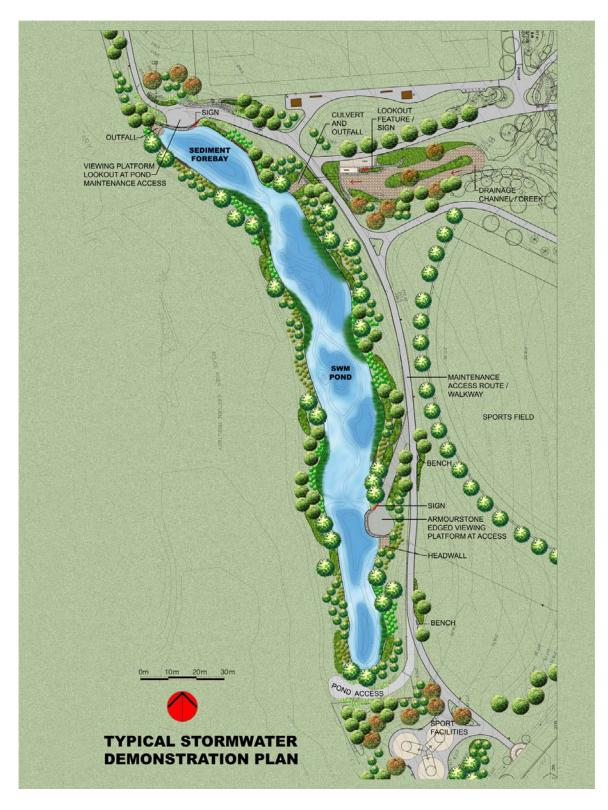
Figure 18: Demonstration Plan – Wet Pond
