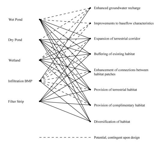
Figure 4 : Potential Stormwater Management Facility Positive Effects
