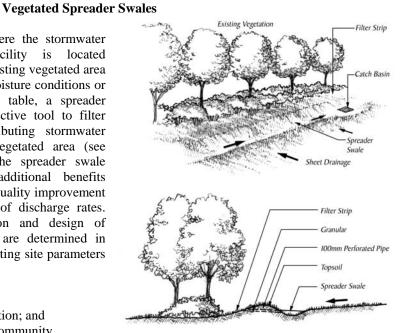
Figure 23: Vegetated Spreader Swale
