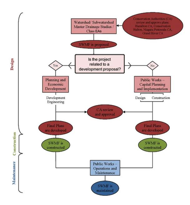
Figure 1 : Stages in Planning and Design of Stormwater Management Facilities (SWMF)
