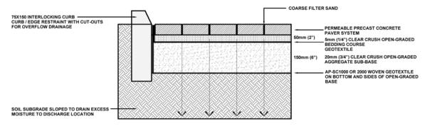
Figure 11: Porous Pavement Detail
