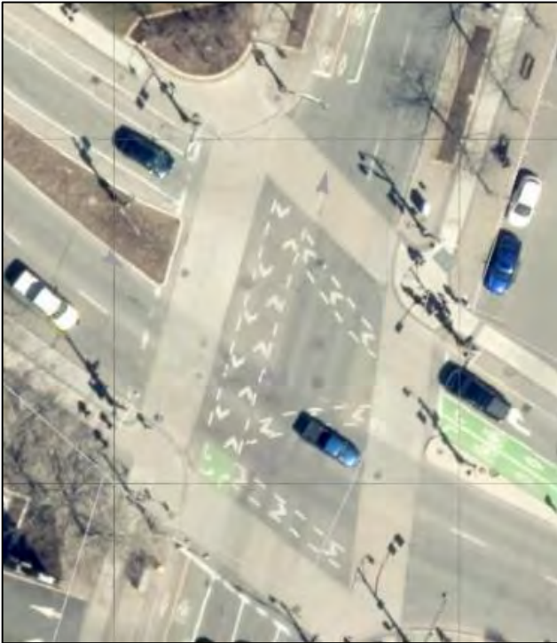
Bay St @ York Blvd, Hamilton Special turning box in intersection
