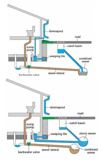
Best Practice recommends that downspouts discharge to the ground surface, and the Foundation Drain should discharge to the ground if the soil conditions permit or connect to the Storm Sewer if available
